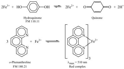
The absorbance of the iron-o-phenanthroline complex is measured with a spectrophotometer. A series of standards of known concentration of the complex are prepared, and a standard curve of absorbance versus concentration is developed to determine the concentration of the complex in the unknown sample. A standard curve of this nature takes advantage of the linear nature of Beer's law:
